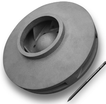
Fig. 1. RBSiC blower wheel made by milling of two semi-finished C-SiC green parts followed by green state joining and subsequent silicon infiltration (courtesy: Schunk Ceramics, Germany).
