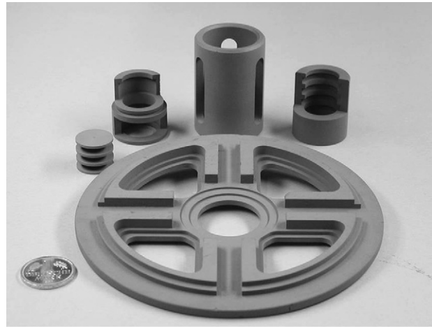
Fig. 5. RBAO “green” parts shaped by high-speed milling and turning. The high strength of the isopressed \text{Al}/\text{Al}_2\text{O}_3 powder compacts allows damage free machining using conventional grips and tools.
