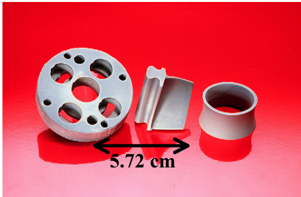
Fig. 4. Parts are made by fused deposition of ceramics (FDC) using a 55 vol.% \text{Si}_3\text{N}_4 powder loaded polymer filament of 1.78 mm diameter. The port plate (on the left) was built by FDC with minimal surface smoothing of the top face before sintering. The blade (middle) is a turbine blade that was green machined by hand after building by FDC and then sintered. The nozzle (right) is a generic nozzle shape for a rocket engine application that was built by FDC without any further machining at the green or sintered state (courtesy: S.C. Danforth, Rutgers Univ., USA, see also ref. [94]).
